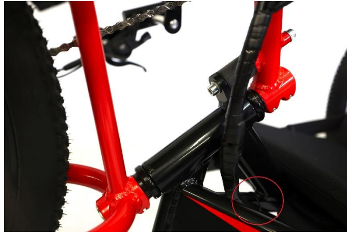
Fig. 24. The wiring attachment point when it comes out from under the seat.
