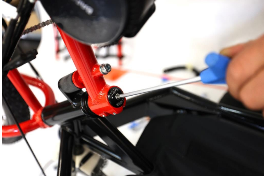
Fig. 6. Steering tube cap mounting screw.
