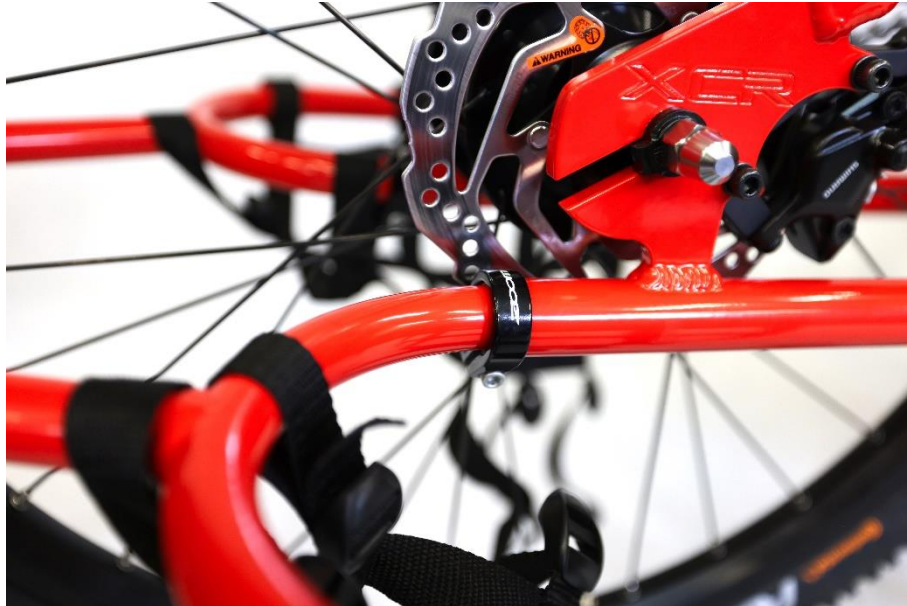
Fig. 15. Footrest pushed in and locked with clamps.
