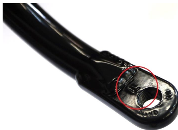
Fig. 9. Crank assembly side marking; the photo shows the left crank.
