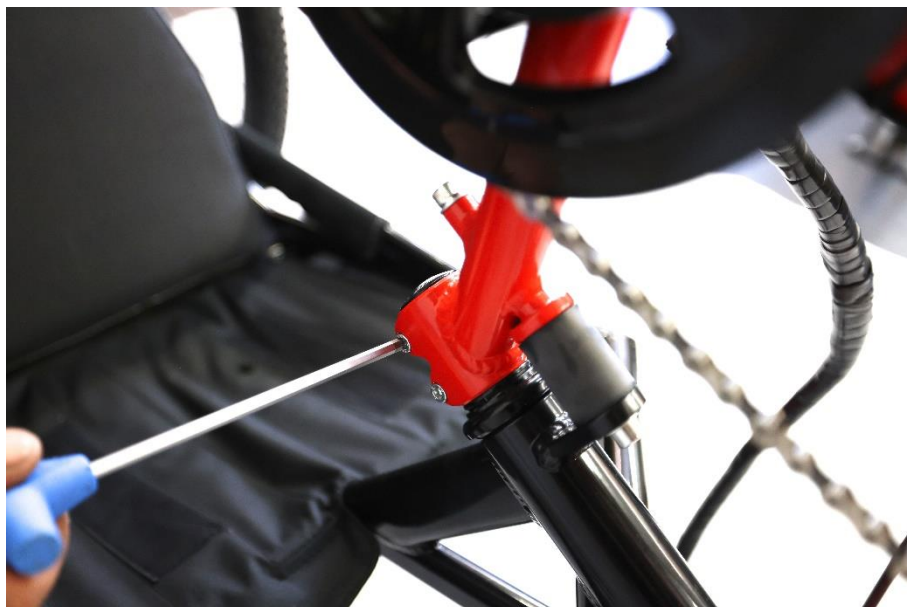
Fig. 7. Tightening the upper arch screws.
