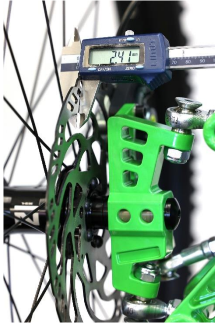
Fig. 27. Method of measuring the brake disc thickness (illustrative photo)
