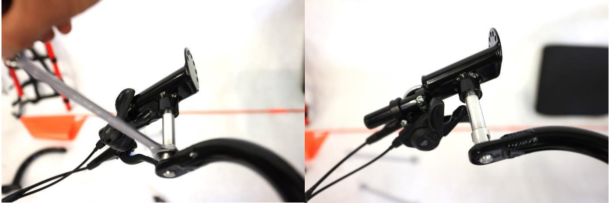
Fig. 13. Mounted right crank grip, left grip has a left-hand thread.
