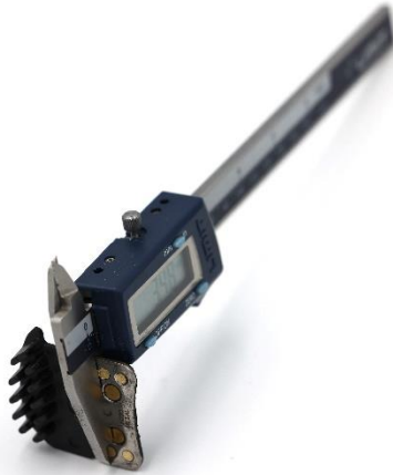
Fig. 28. Method of measuring the brake pad lining thickness
