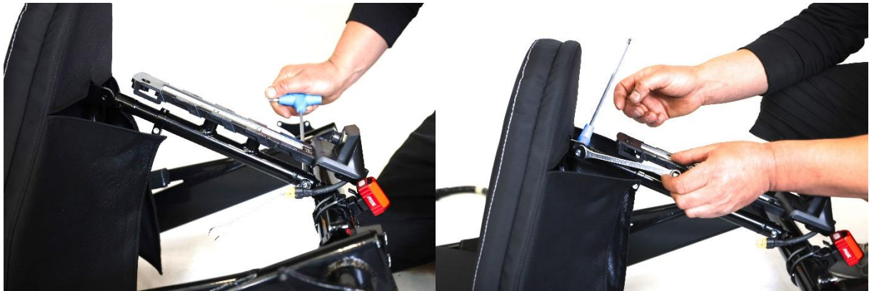
Fig. 17. Installing the backrest support with the battery base.
