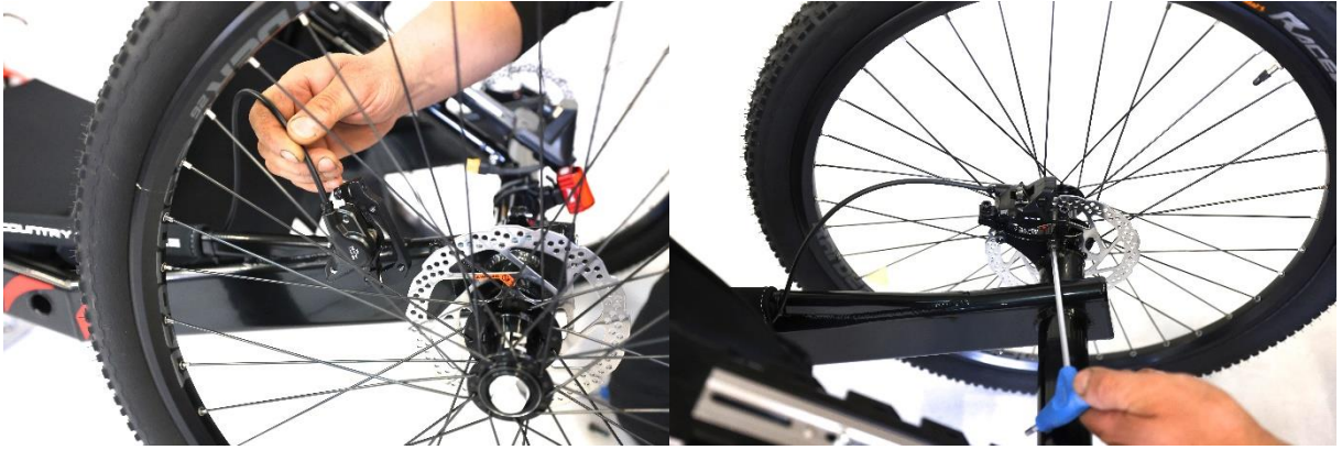
Fig. 22. Rear brake caliper assembly.
