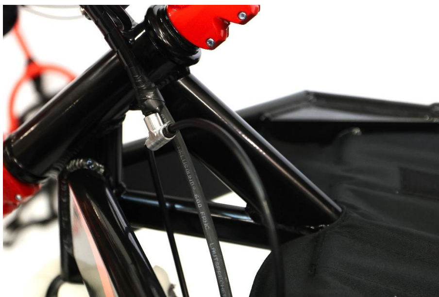
Fig. 19. Wiring bundle with T-piece and rear caliper brake lines
