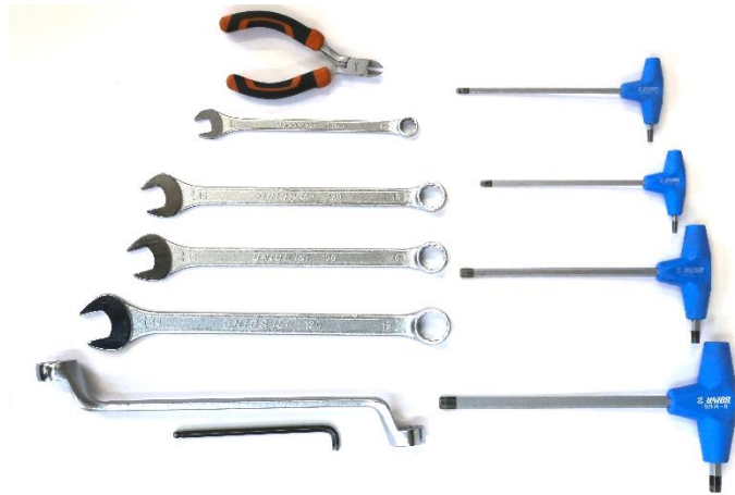
Fig. 2. The set of tools necessary for assembling the handcycle
