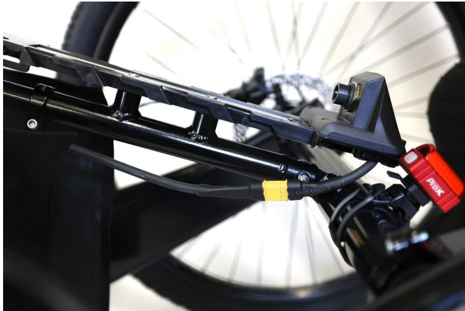
Fig. 23. Connecting the electrical system to the battery base.
