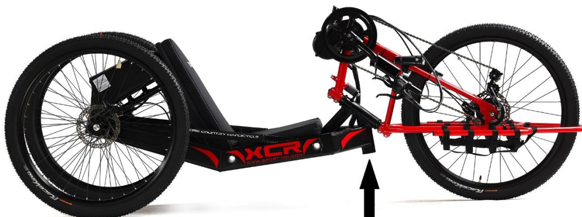
Fig. 31. Place an object here to check the headset slack.
