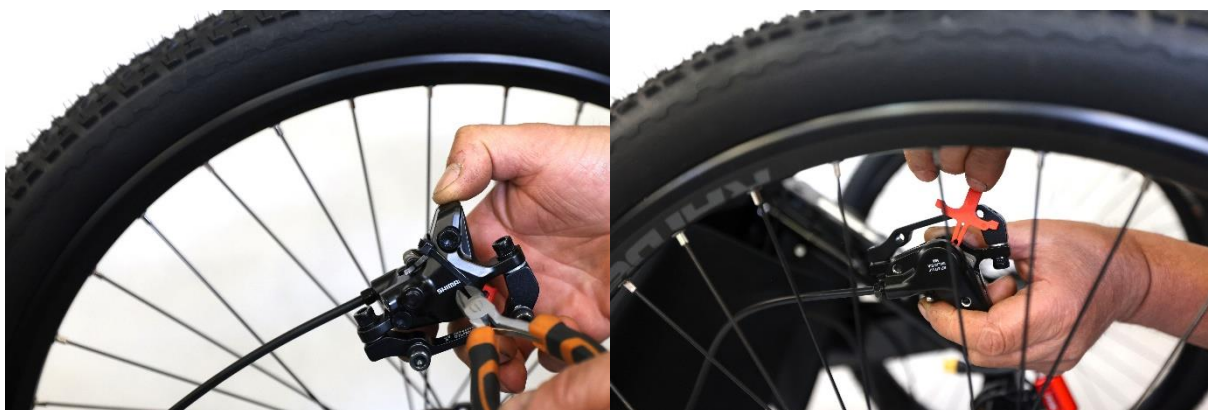
Fig. 21. Removing the spacers from between the brake pads.
