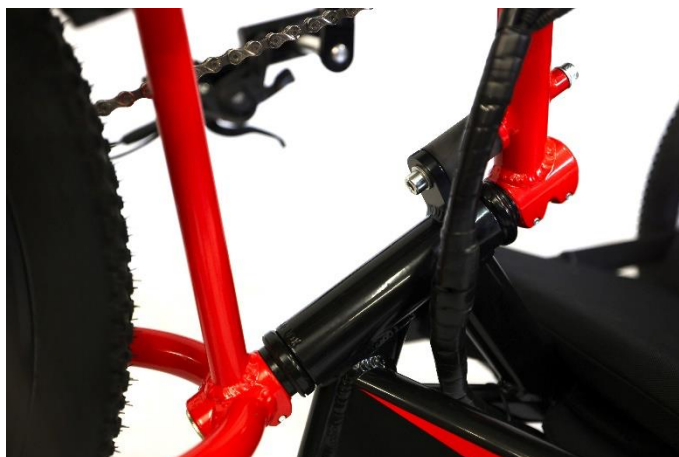
Fig. 20. Routing the wiring bundle with brake and electric cables
