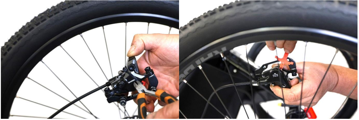
Fig. 22. Removing the spacers from between the brake pads.
