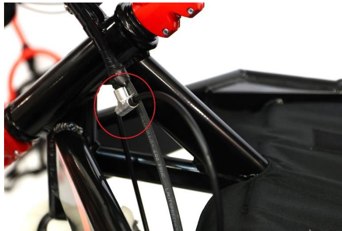
Fig. 20. Wiring bundle with T-piece and rear caliper brake lines (photo shows XCR handcycle; similar solution was used in Troublemaker)
