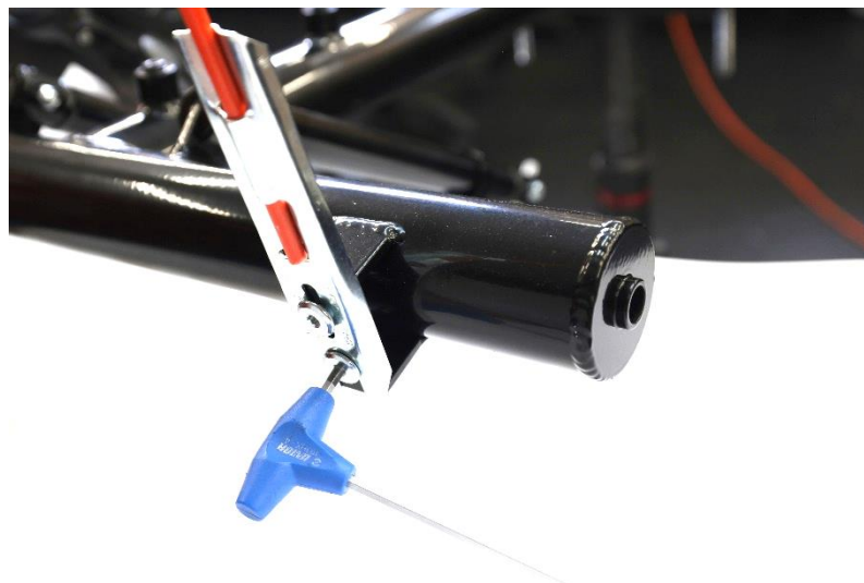
Fig. 25. Flag assembly (the right side is shown in the photo, the left side has similar assembly)
