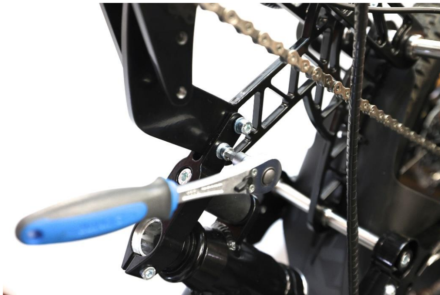
Fig. 6. Screws connecting the upper arch to the fork.
