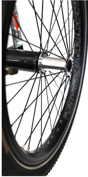
Fig. 18. Fig. 18. Correctly attached rear wheel
