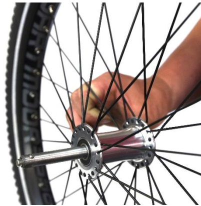
Fig. 17. Handcycle rear wheel axle with the quick-release skewer
