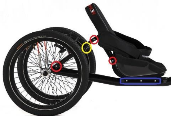
Fig. 27. Screws that need to be loosened to adjust the distance between the seat and the drive cranks.
