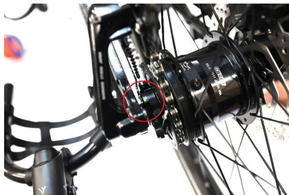
Fig. 33. Location of calibration marks on the hub selector
