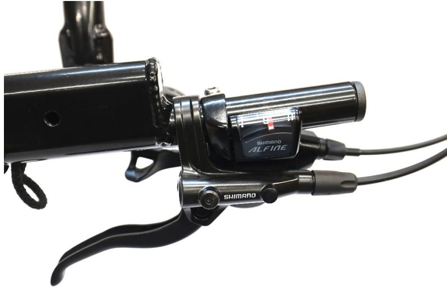
Fig. 32. Setting gear no. 6 in Alfine 11
