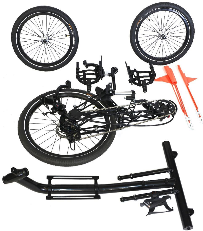
Fig. 1. Components of the Troublemaker handcycle included in the package (the seat and the backrest attached to the frame are not visible in the photo).
