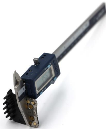
Fig. 31. Method of measuring the brake pad lining thickness
