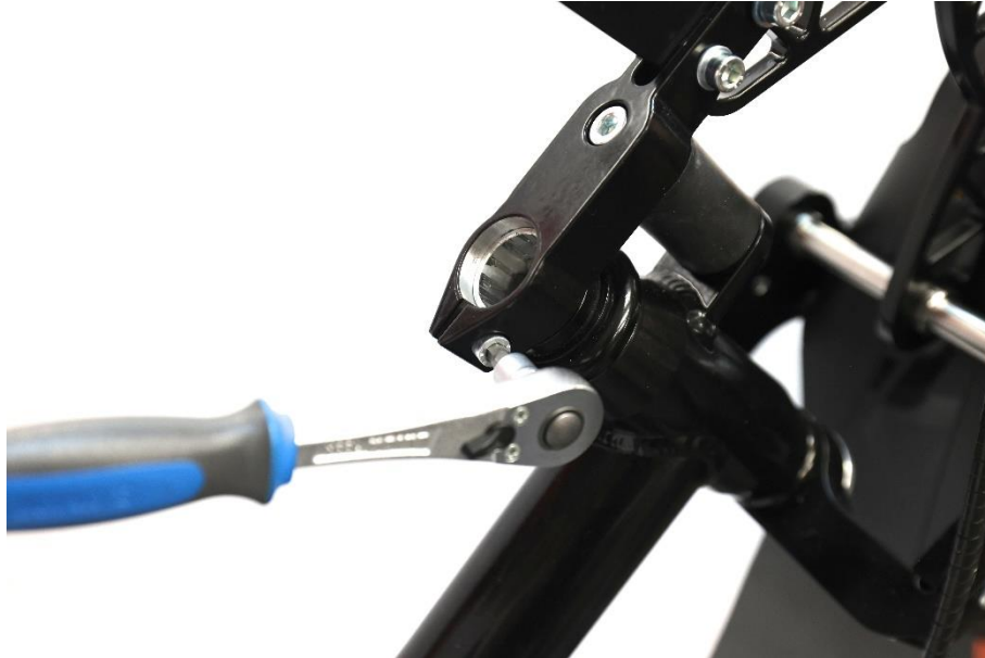
Fig. 5. Tightening the upper arch clamp screw.
