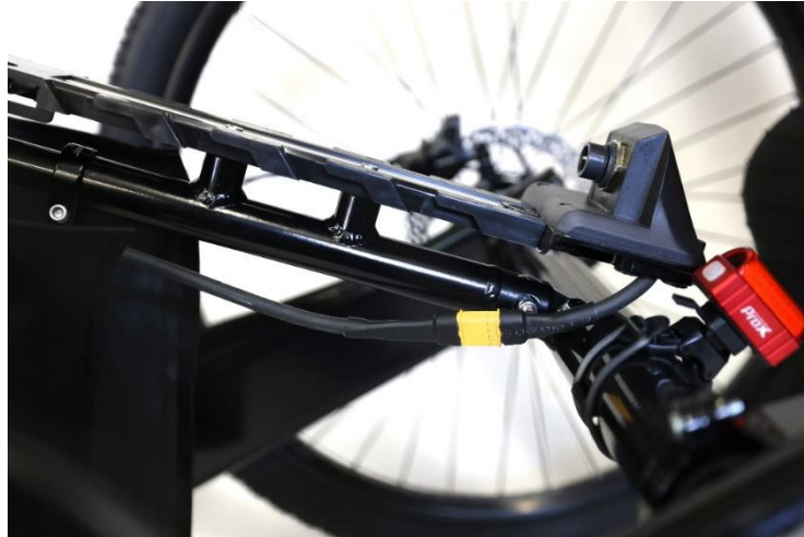
Fig. 24. Connecting the electrical system to the battery base (the photo shows an XCR handcycle; in Troublemaker, the connection looks identical, but the base is mounted in the opposite direction).
