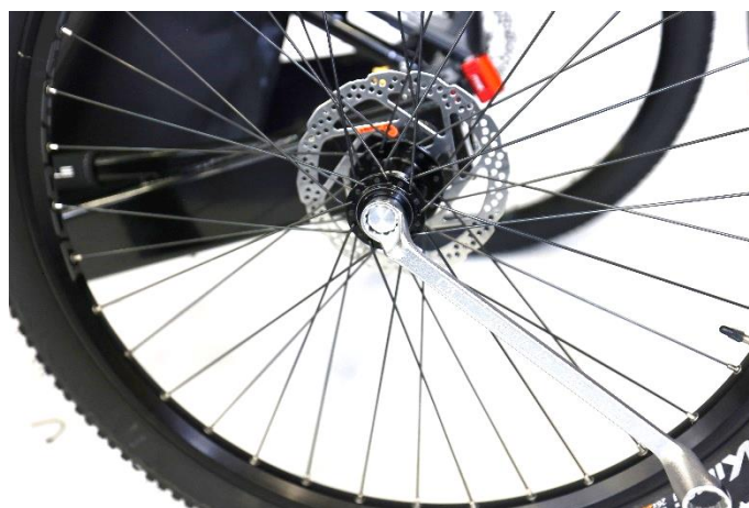
Fig. 19. Rear wheel assembly (the photo shows the XCR handcycle wheel; the assembly in Troublemaker is similar)
