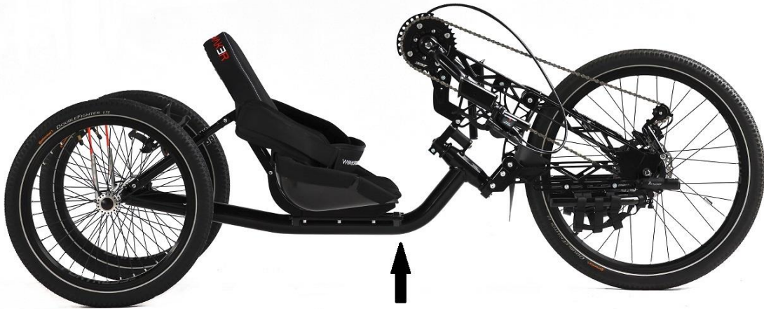
Fig. 36. Place an object here to check the headset slack.
