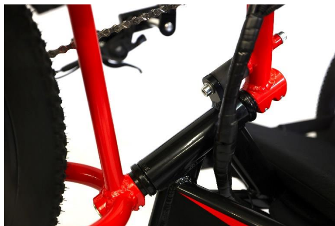
Fig. 21. Routing the wiring bundle with brake and electric cables (the photo shows an XCR handcycle; a similar solution was used for Troublemaker)
