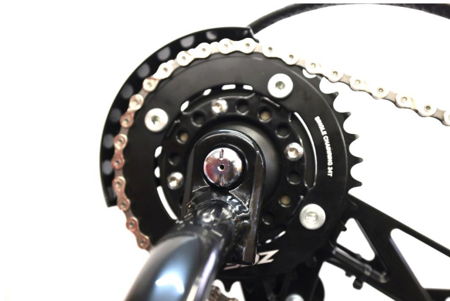
Fig. 13. The final result of mounting the drive crank on the Schlumpf gear.
