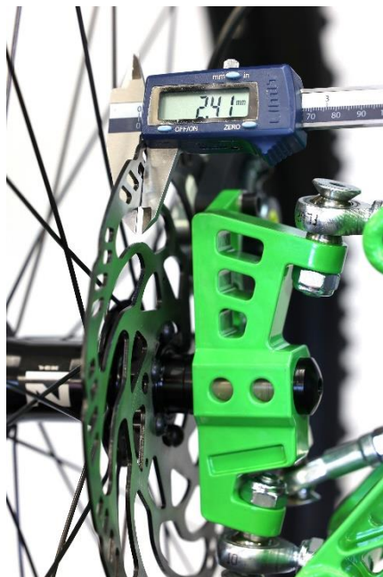
Fig. 30. Method of measuring the brake disc thickness (illustrative photo)
