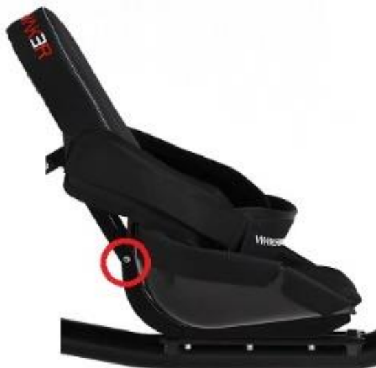
Fig. 16. Bolt connecting the backrest profile with the seat profile (here visible on the right side of the handcycle)
