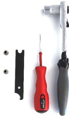
Fig. 10. Set of tools for assembling the cranks on a Schlumpf Mountain Drive
