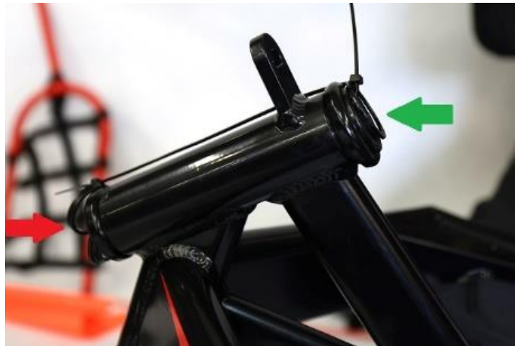
Fig. 2. Frame head with a headset (photo shows fork head in XCR handcycle with similar bearings).
