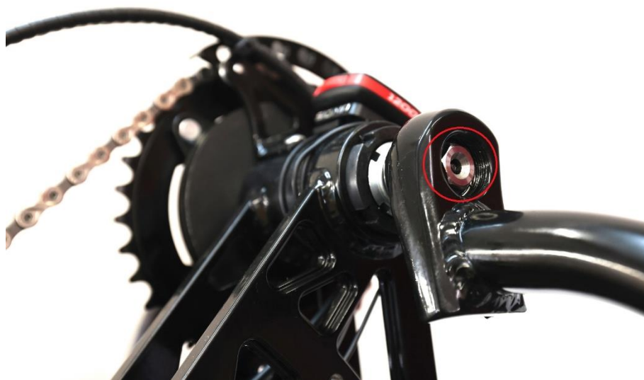
Fig. 11. Crank mounting screw marked with a red loop.
