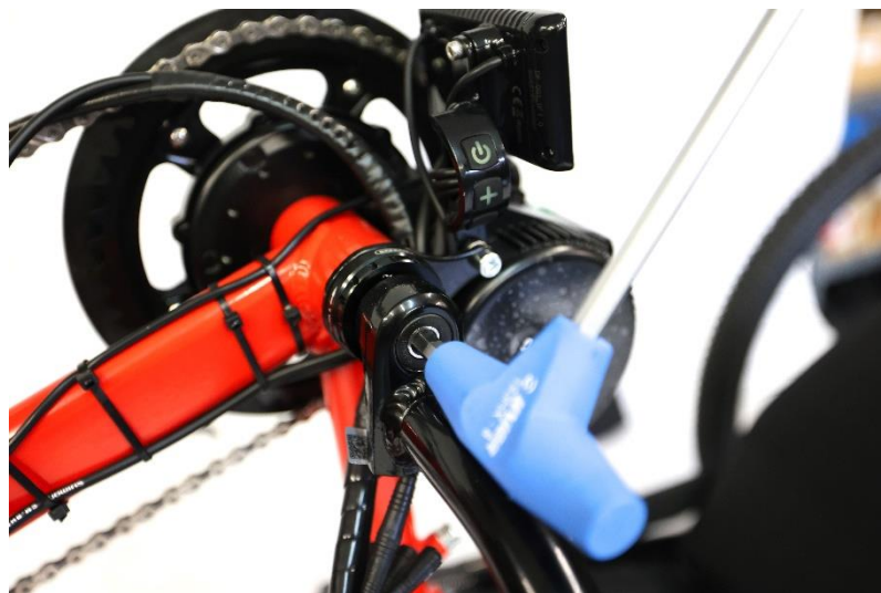
Fig. 9. Crank assembly with electric assist option (photo shows the XCR handcycle. For Troublemaker, the assembly is identical)
