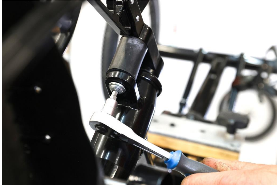
Fig. 7. Lower steering limiter mounting screw.
