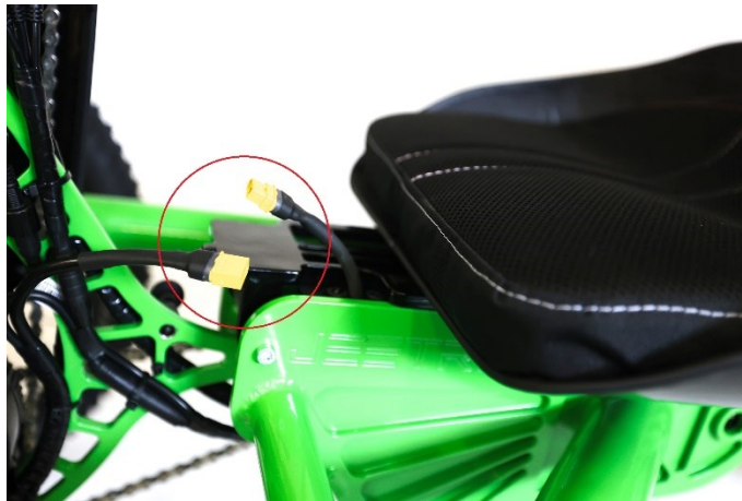
Fig. 12. Connecting the socket and plug after installing the battery
