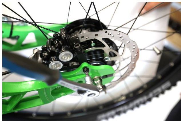
Fig. 14. Attaching the rear brake caliper
