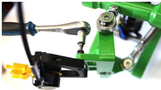
Fig. 23. Mounting the front brake caliper
