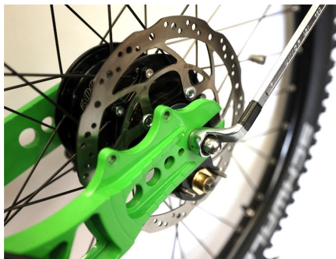
Fig. 7. Attaching the rear wheel to the wishbone hooks
