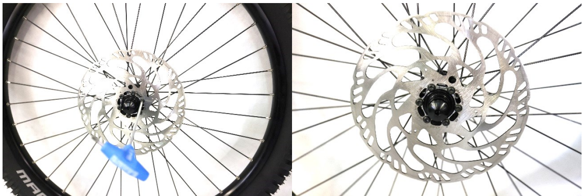
Fig. 3. Attaching the brake disc to the wheel hub
