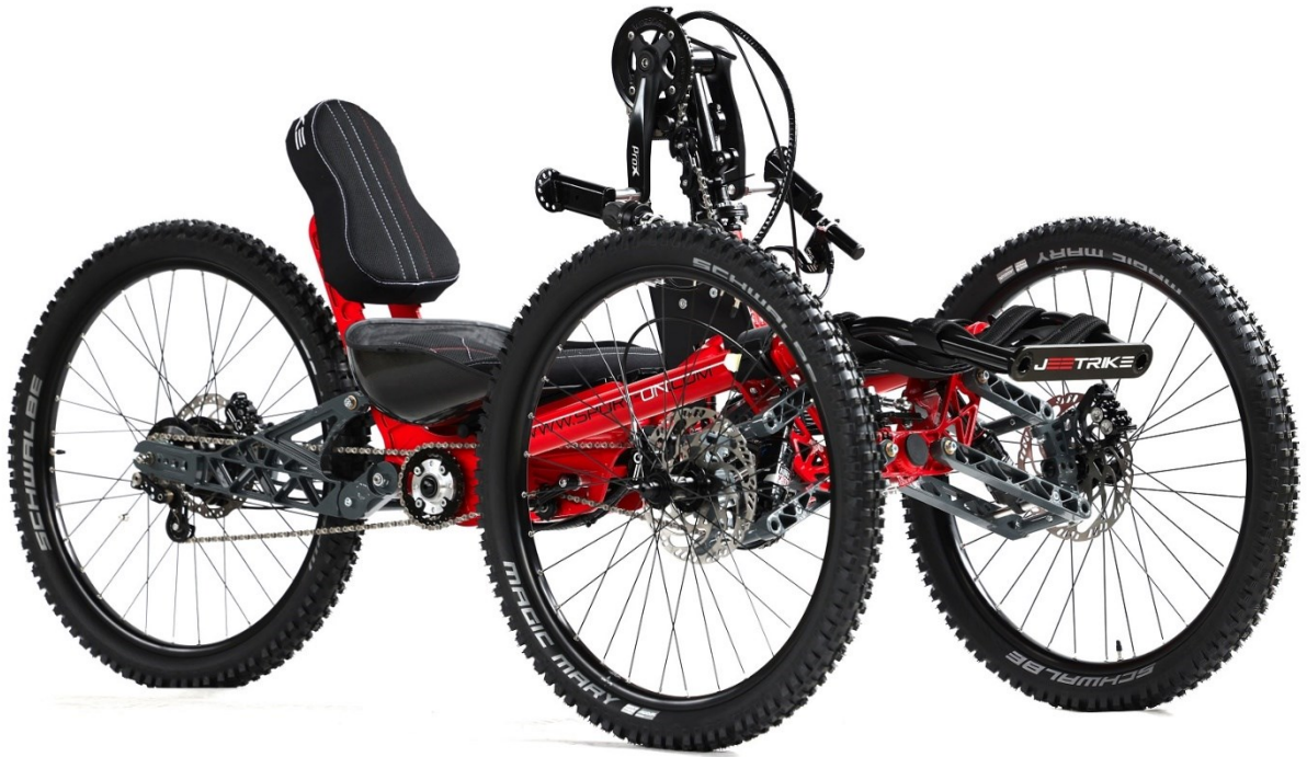
Fig. 28. The final result - the complete Jeetrike handcycle
