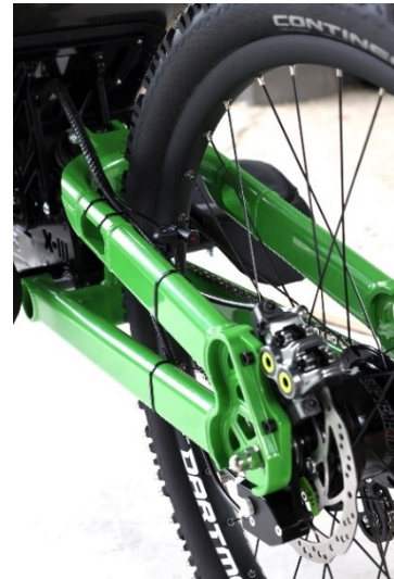
Fig. 19. Location of the selector in relation to the hub and wishbone after completing the connection (example shown: Explorer III)
