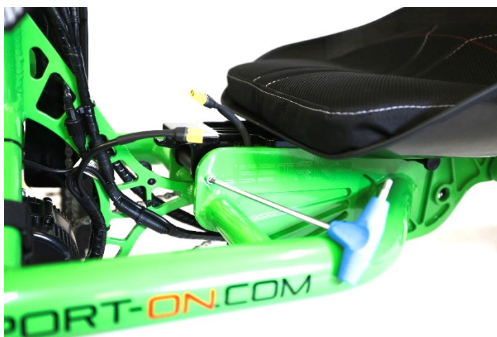
Fig. 9. Mounting the seat - attaching the seat rotation axis on the handcycle frame
