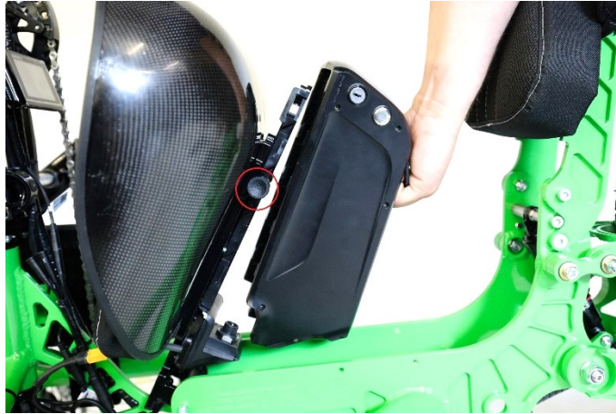
Fig. 11. Battery installation method
