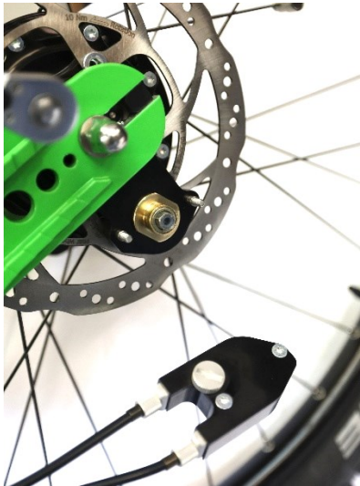
Fig. 18. Gear selector before connecting to the hub mechanism
