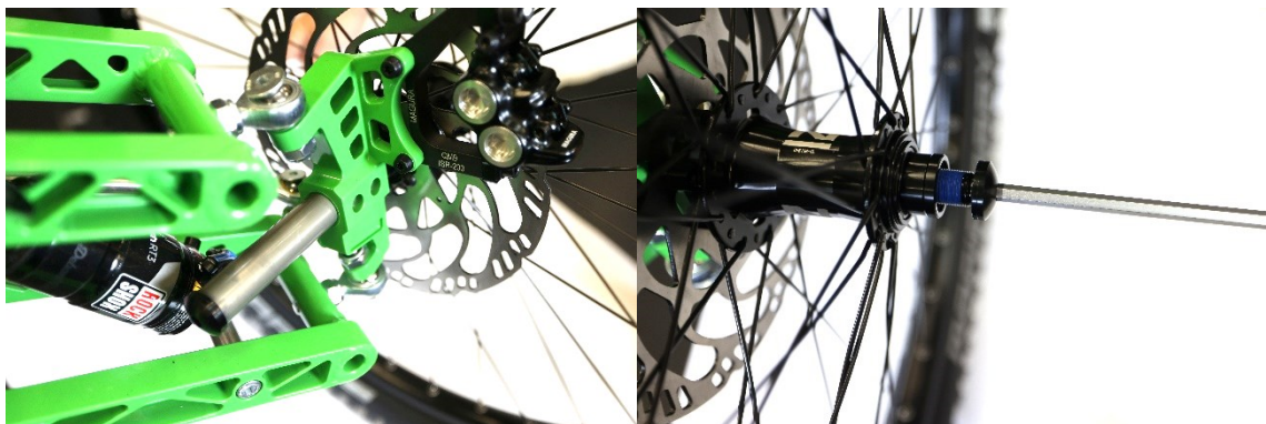
Fig. 24. Front wheel assembly – left: the steering knuckle side, right: the outer side
