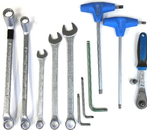
Fig. 2. The set of tools necessary for assembling the handcycle
