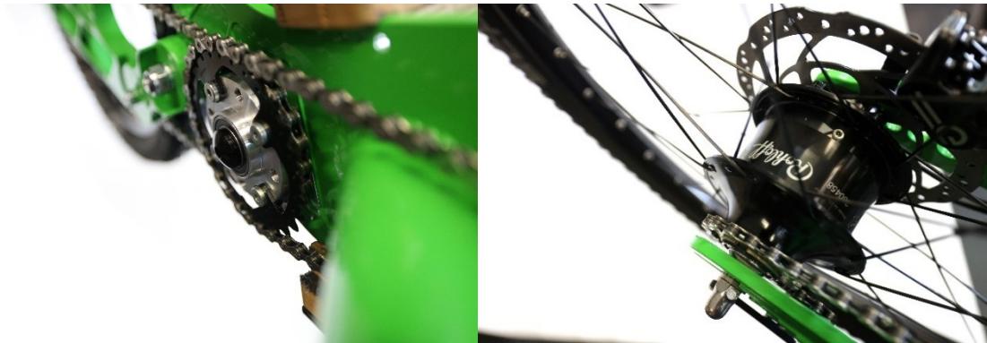
Fig. 21. Threading the rear chain - intermediate gear on the left, rear hub chainring on the right
