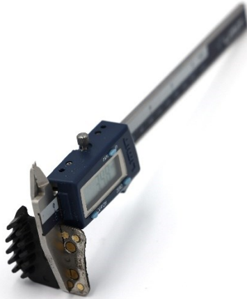
Fig. 30. Method of measuring the brake pad lining thickness
