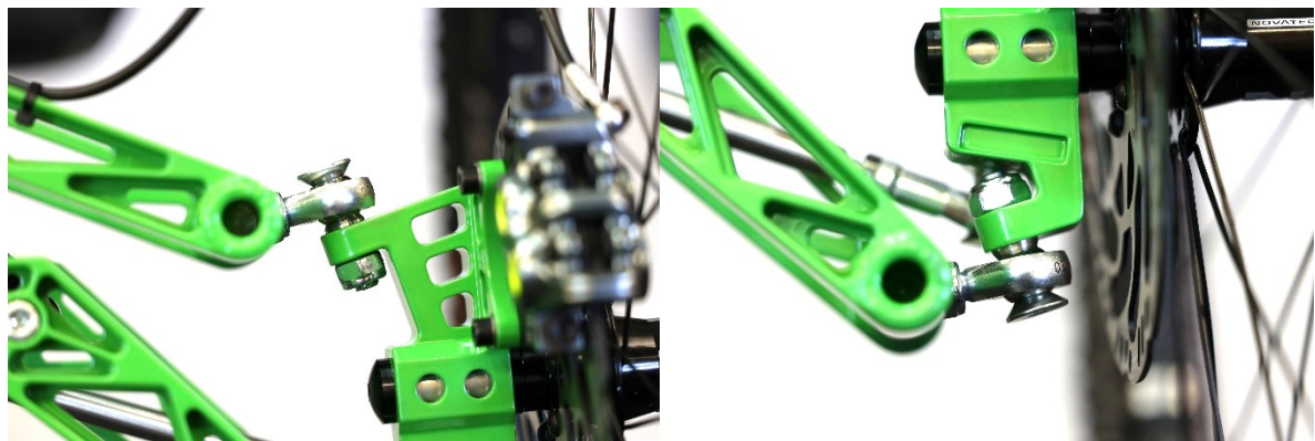
Fig. 35. Joints connecting the wishbones with the steering knuckle: the upper joint on the left, the lower joint on the right
