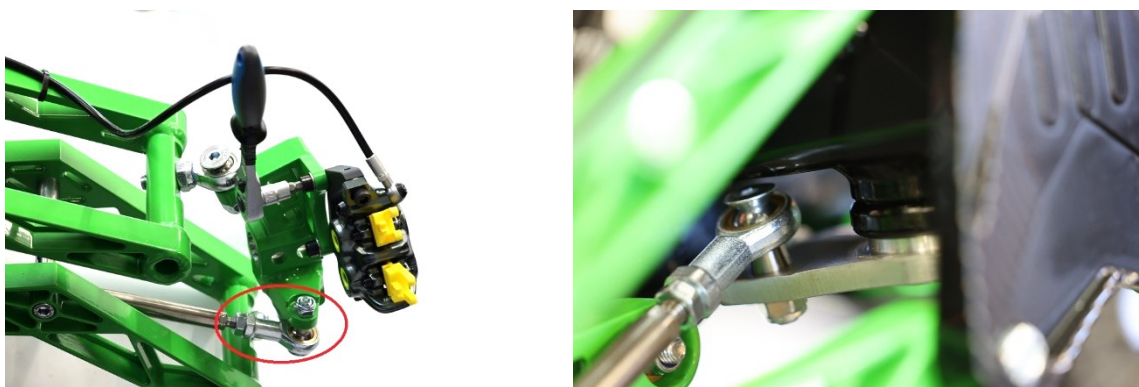
Fig. 33. Steering handle joints: external on the left, internal on the right
