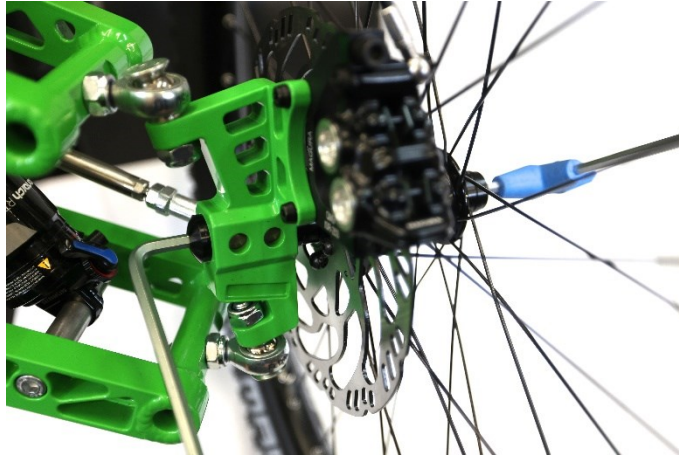
Fig. 25. Front wheel assembly - tightening the screws
