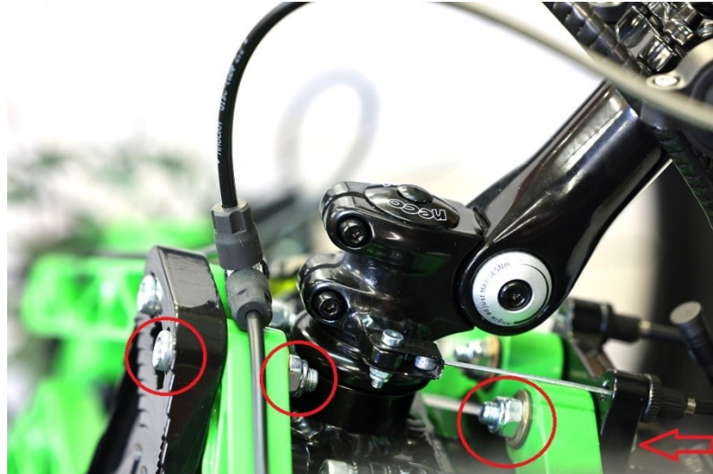
Fig. 34. Bolts connecting the upper wishbone to the frame
