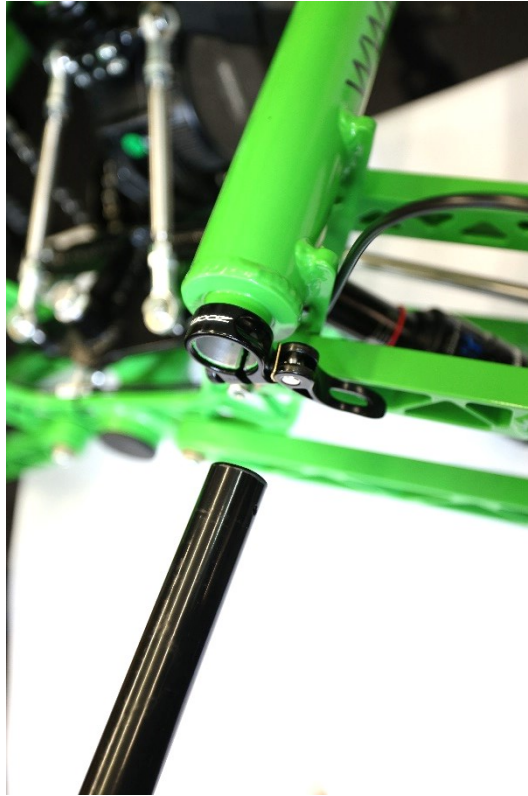
Fig. 27. Footrest socket with the clamp visible
