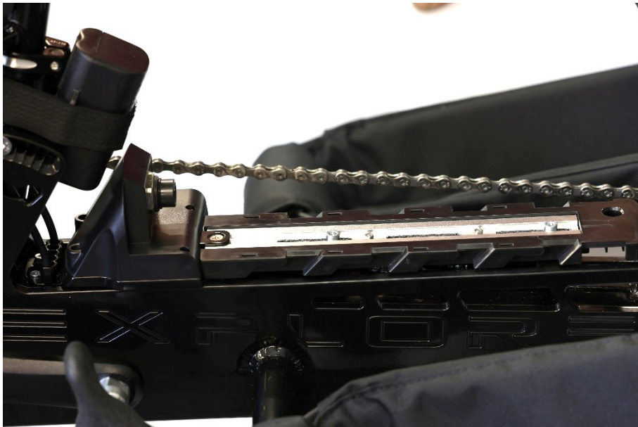
Fig. 25. Attached base with the cable placed underneath
