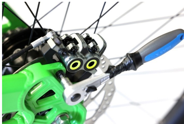
Fig. 10. Attaching the rear brake caliper
