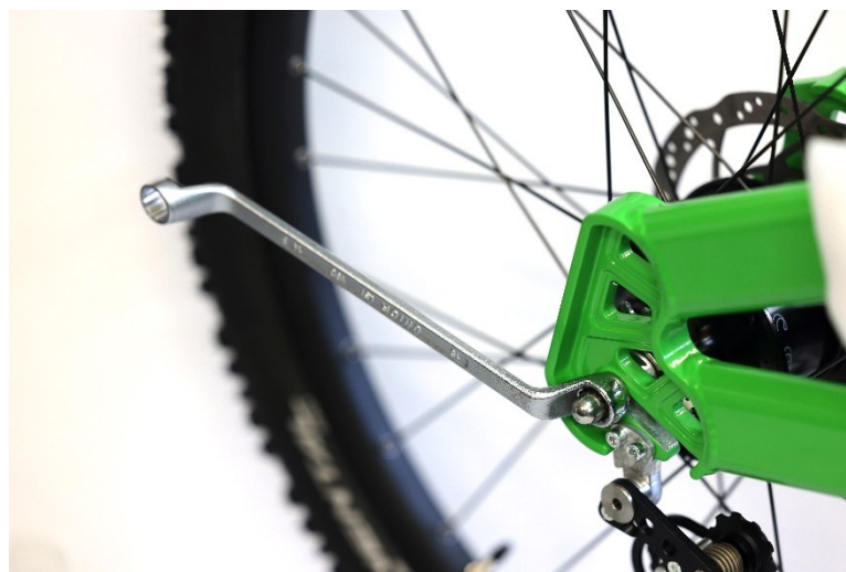
Fig. 7. Attaching the rear wheel to the wishbone hooks
