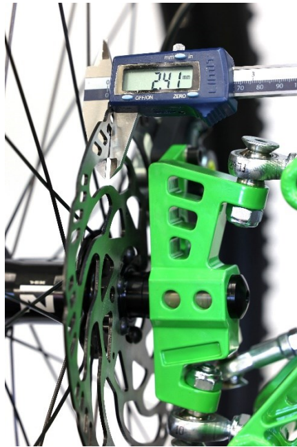
Fig. 28. Method of measuring the brake disc thickness
