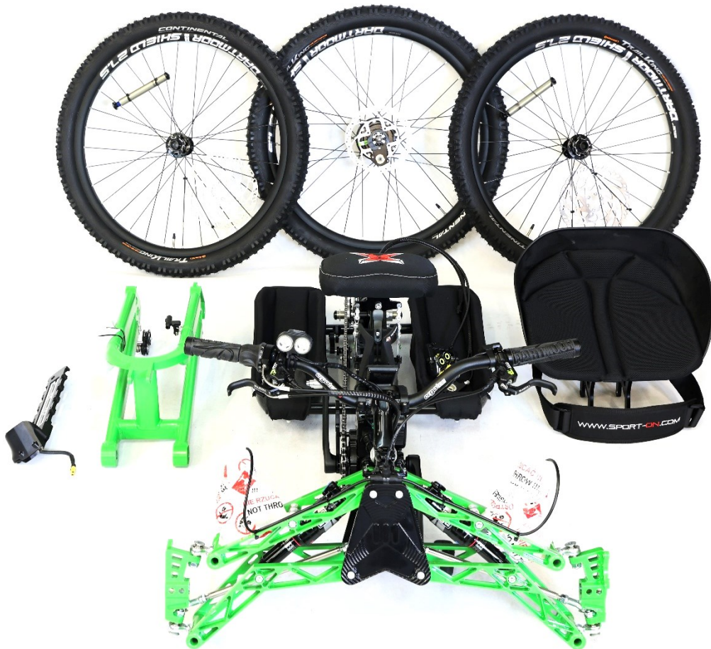
Fig. 1. Components of the Explorer handcycle included in the package
