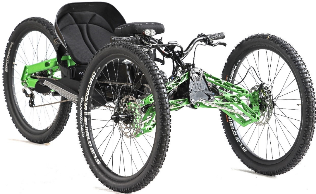
Fig. 26. The final result - the complete Explorer handcycle
