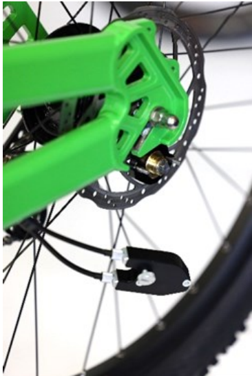
Fig. 14. Gear selector before connecting to the hub mechanism
