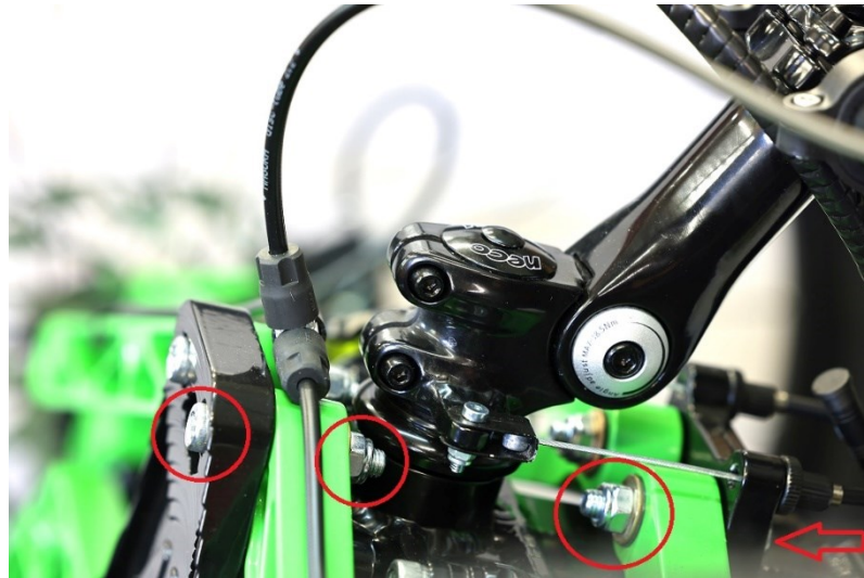
Fig. 35. Bolts connecting the upper wishbone to the frame
