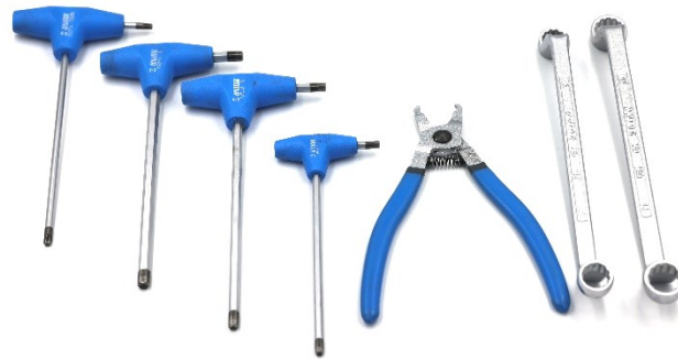
Fig. 2. The set of tools necessary for assembling the handcycle
