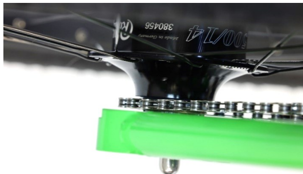
Fig. 16. Threading the rear chain (the inner chainring is smaller)
