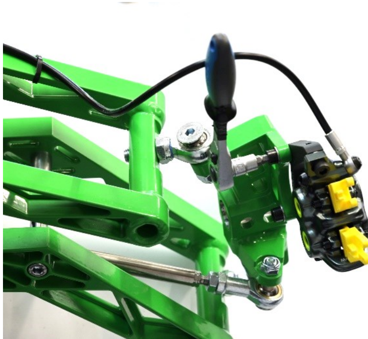
Fig. 21. Mounting the front brake caliper
