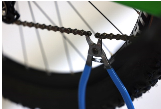
Fig. 19. Fastening the rear chain connecting the intermediate gear with the rear hub
