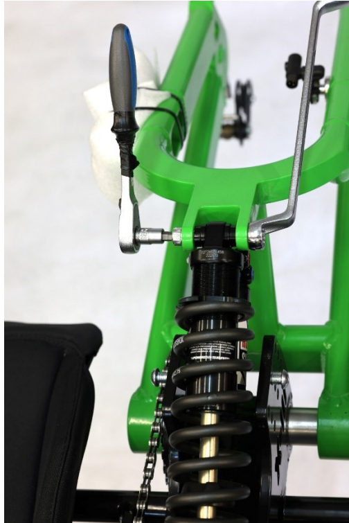
Fig. 6. Threaded connection of the rear suspension shock absorber axis with mounting points in the wishbone
