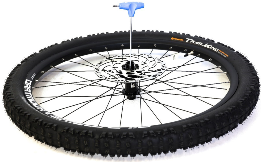
Fig. 3. Attaching the brake disc to the wheel hub
